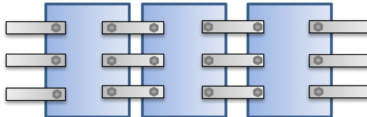
In every case shown, the combination of the jar's internal resistance and its connection resistances forms a "loop" of resistances that gets multiplied by the number of jars in the string. A partial view of the loop resistances in a string of jars is shown below:
