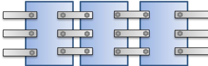
In every case shown, the combination of the cell's internal resistance and its connection resistances forms a "loop" of resistances that gets multiplied by the number of cells in the string. A partial view of the loop resistances in a string of cells is shown below:
